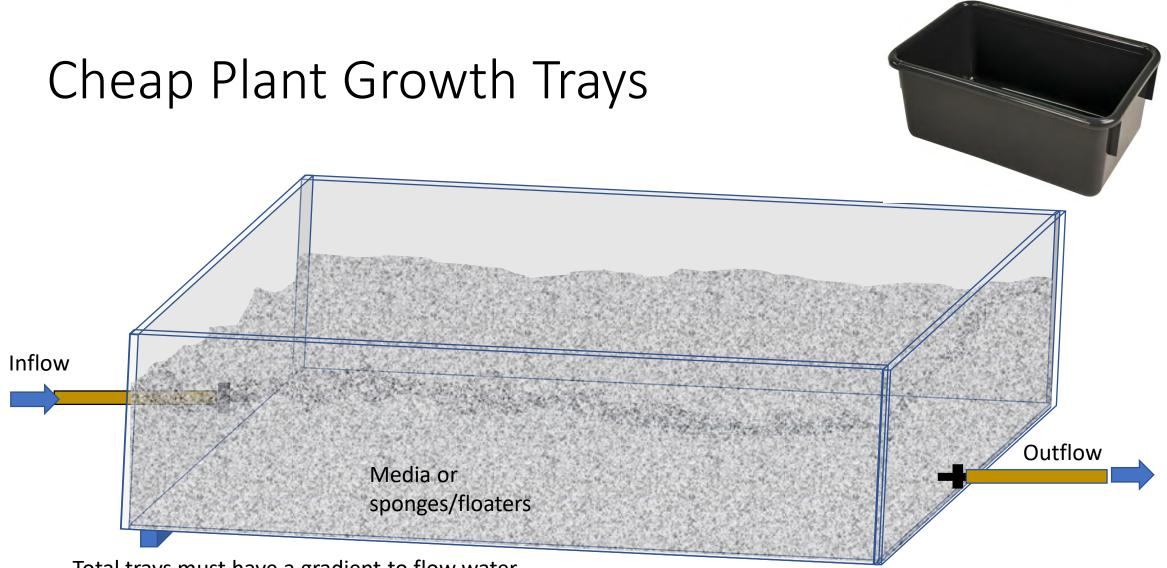
Total trays must have a gradient to flow water
