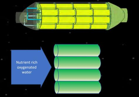
Note : for free flowing algae, pumps must not use impellers (i.e. be fluidic pumps or slow stirrers)
